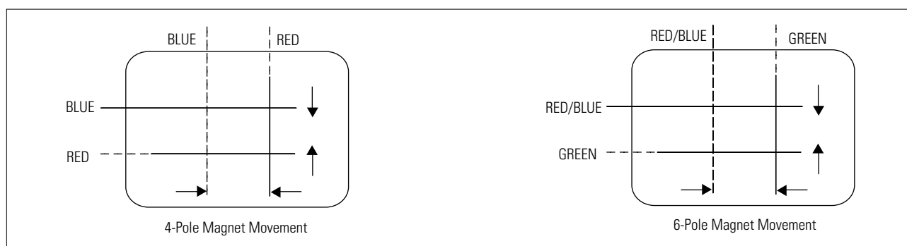
Fig. 4-5 Center Convergence Adjustment
